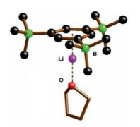
The attachment of three negatively charged trihydridoborate or trimethylborate substituents to a benzene ring leads to the formation of  ${\rm Li}^+{-}\pi$  complexes even in the presence of competing THF or 12-crown-4 ligands.
