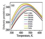
A new oxide, Bi<sub>2</sub>La<sub>0.5</sub>Sr<sub>0.5</sub>Nb<sub>1.75</sub>Sc<sub>0.25</sub>O<sub>9</sub> (I), crystallizes in the polar  $A2_1am$  space group at room temperature. The relaxor behavior of I was characterized by using dielectric, piezoelectric, and ferroelectric measurements. The relaxation parameter  $(\gamma)$ , piezoelectric coefficient  $(d_{33})$ , and remanent polarization  $(P_T)$  for I are 1.91, 3 pC/N, and 5.7  $\mu$ C/cm<sup>2</sup>, respectively.
